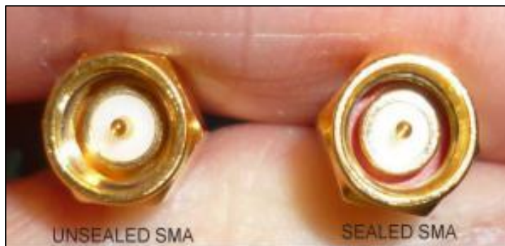
Figure 3 - Unsealed vs Sealed SMA Connectors
